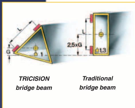
*Global's TRICISION extruded triangular cross section bridge beam enhances dimensional stability for superior metrology performance.*
