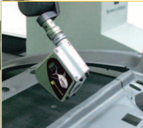
**The CMM-V high-resolution camera** gives you measurement performance that a tactile probe alone literally can't touch. With the CMM-V, your Global CMM will be ideally suited for a wide range of parts that require non-contact measurement —
