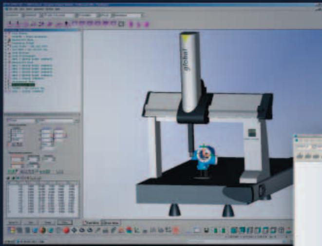
*PC-DMIS software takes full advantage of Global scanning capability. In the example shown, the machined flange surface is being scanned for flatness; PC-DMIS allows for the specification of scan paths, shown as the yellow curvilinear line below.*
